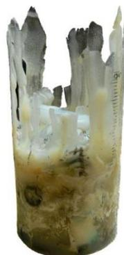
During a process, syringes are melted and sterilized to form a compact recyclable plastic puck. This puck remains in the sharpsCAN™. The sharpsCAN™ is a recyclable container.
